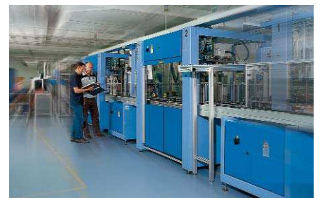
Fully automated rotor production line with 100% process monitoring
